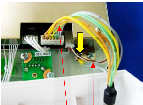
Box cable Cable for LCD inverter (red/white)
